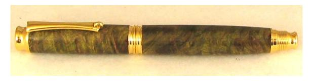
Needed: Mandrel-A **Bushing Set-38A** Drills-15/32, 25/64 Blank Size- 5/8" x 5/8"
